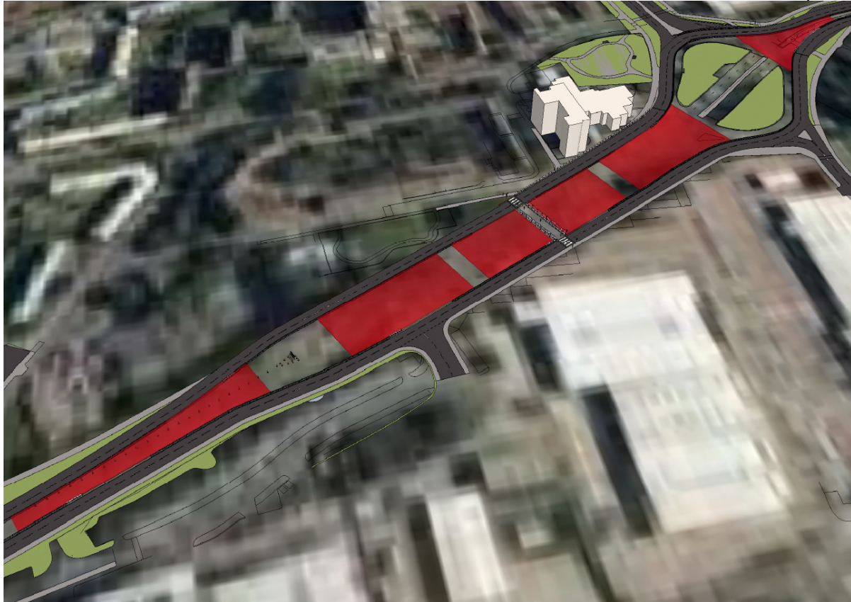
Figure 5 Example of loss of works area due to TVCB specification at an at-grade pedestrian crossing
